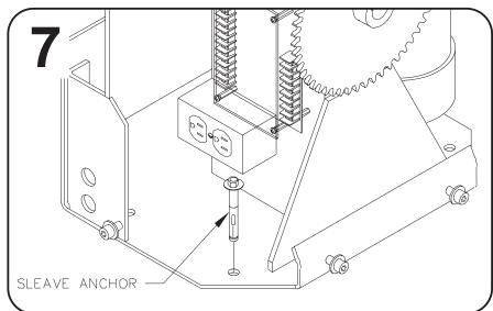
O When the gate operator is correctly positioned on the concrete surface or pad, mark the base hole locations onto the cement with a felt tip marker or equivalent. Once marked, move the operator to the side and drill the 4 holes using a 3/8" masonry bit. Place the operator back into position. Insert the four sleeve anchors into the holes and firmly tighten.
